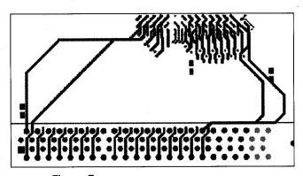
Figure 7—Lines expanded to match longest routed length
