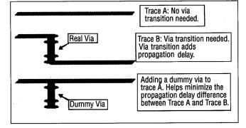
Figure 9—Example of adding a "dummy" via to a trace
