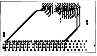
Figure 6—Routing outside lines before length-matching to longest line
