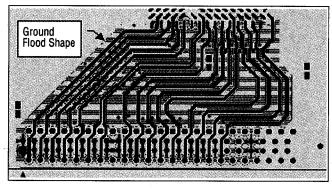
Figure 10—Routed RDRAM channel with ground flood shape
