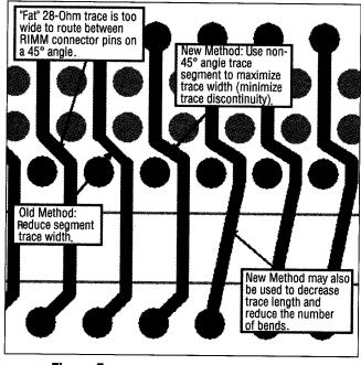
Figure 5—Using non-45° angles to minimize line discontinuities
