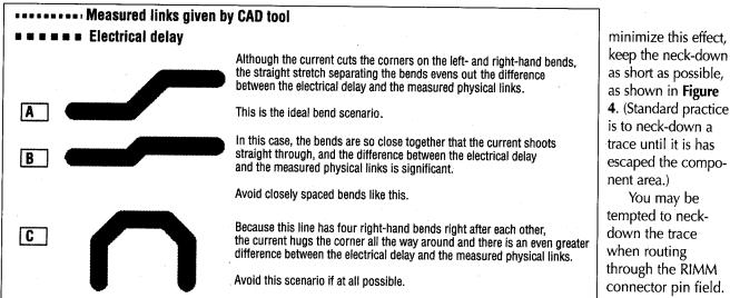
Figure 3—Example of current cutting the corner on bends
